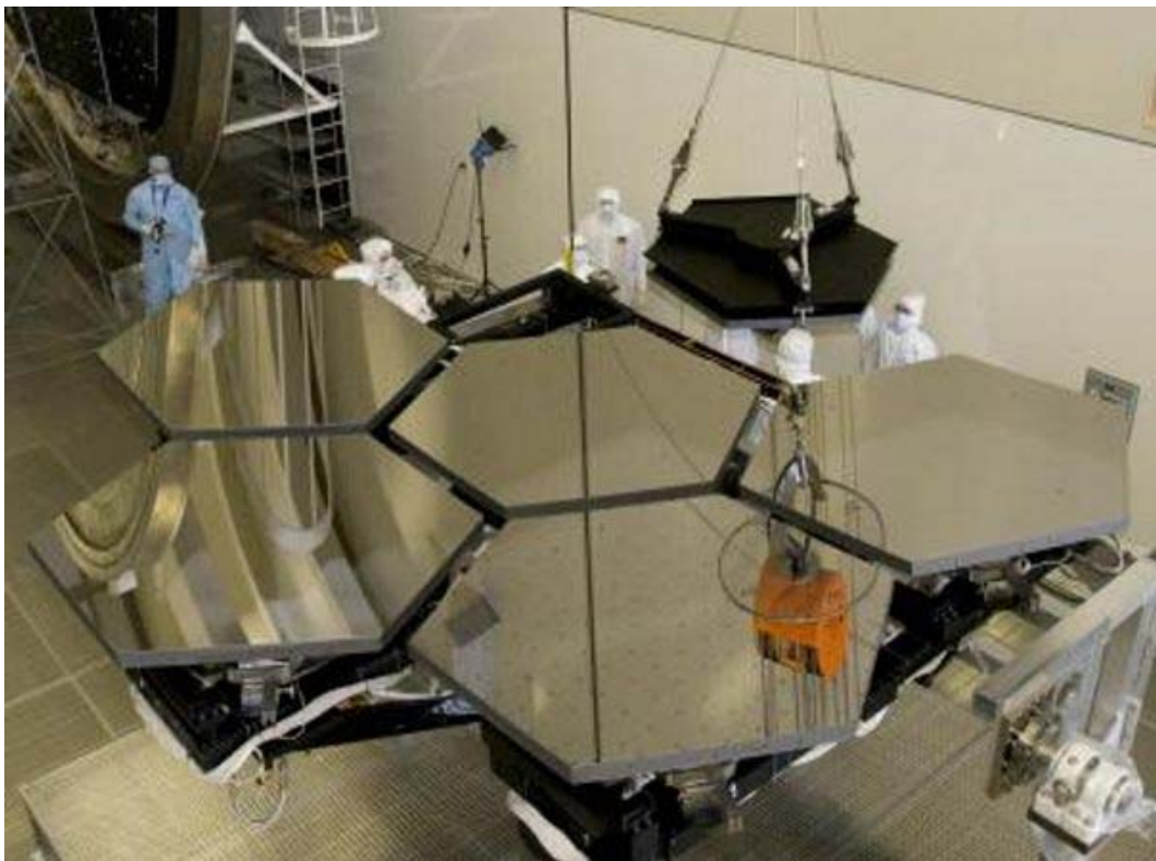
JWST Primary Mirror Segments being prepared for optical cryo-testing.
