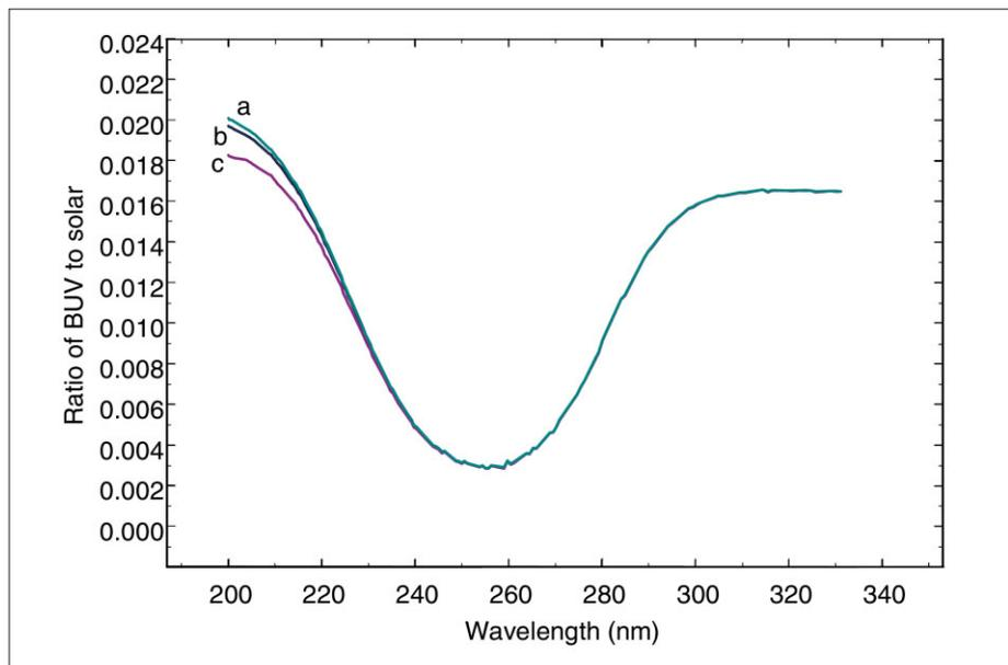
Fig. 8. Modtran computations for nadir geometry. Solar zenith angle  $60^\circ$ , ozone total abundance  $5 \mu\text{-atm}$ . A possible effect of  $\text{H}_2\text{O}_2$  is considered: no  $\text{H}_2\text{O}_2$  (curve a);  $\text{H}_2\text{O}_2$  column of  $2 \times 10^{16} \text{ cm}^{-2}$  (curve b) and  $2 \times 10^{17} \text{ cm}^{-2}$  (curve c).
