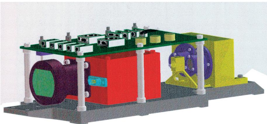
Fig. 5. The AOTF IR channel. From right: entrance lens, AOTF crystal and the two detectors, with the electronics board on top.
