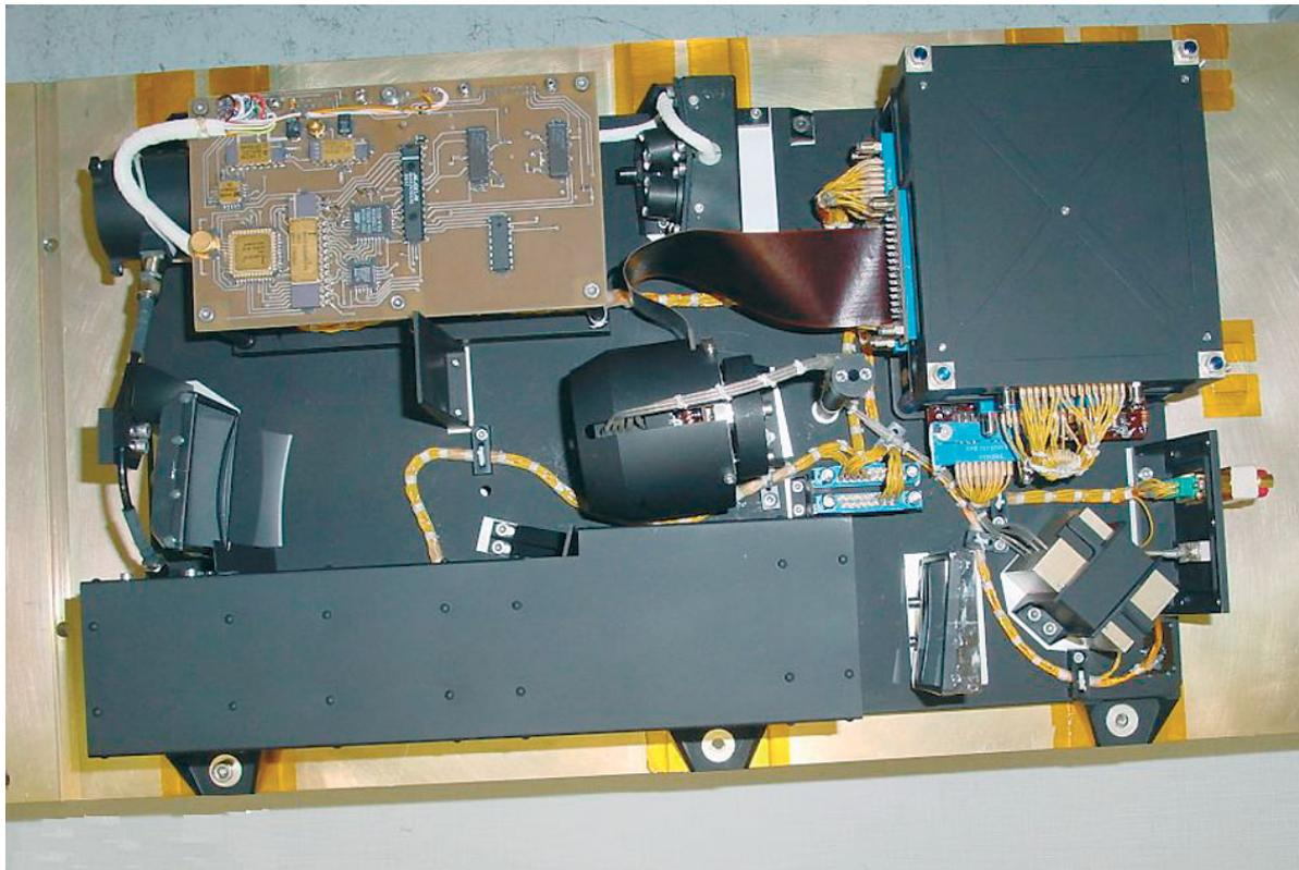
**Fig. 1. Flight Model Sensor Unit of SPICAM** viewed from above. The IR AOTF spectrometer is at top; the UV spectrometer is at bottom. The common optical axis points to the left. For the UV spectrometer, the light enters the mechanical baffle (black), is focused by a parabolic mirror (bottom right) through a slit, then dispersed by the grating (middle left), to be refocused on the intensified CCD Detector (at centre).
