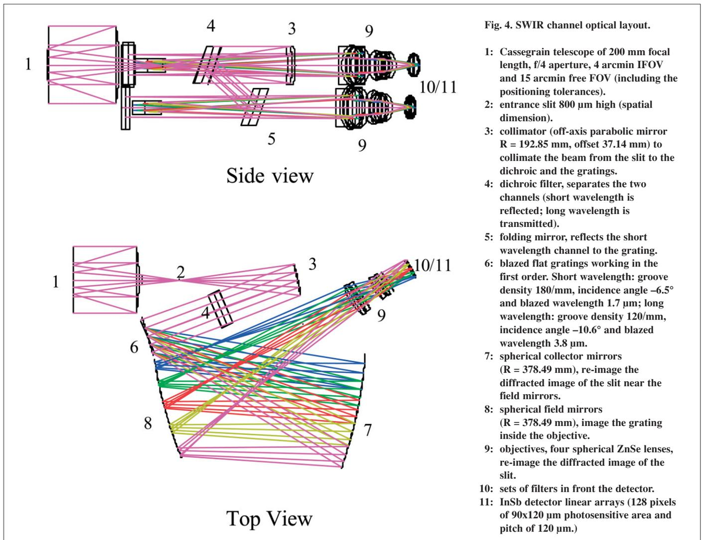
reflective system, then a field mirror and a refractive refocusing system that gives a large aperture on the detection block (f/1.6). It images the spectrum on to a 128-element InSb linear array, cooled to  $< 80\text{K}$ , and multiplexed by a charge transfer device. Sets of filters are implemented in front of the detector to reject the contribution of other orders from the grating.
