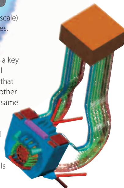
The LFI consists of a cold front-end in the focal plane, linked by rigid waveguides to a warm unit located in the Service Module
