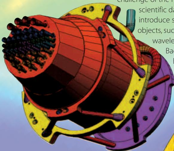
**The High Frequency Instrument (HFI)** is an array of 50 so-called 'bolometric' detectors, which work by converting radiation to heat. They are operated at  $-272.9\text{ }^{\circ}\text{C}$ , a temperature only one tenth of one degree above absolute zero. The HFI detectors will gather data in six wavelength channels between three mm and one third of a mm. The instrument is being built by a Consortium of more than 20 institutes, led by the Institut d'Astrophysique Spatiale in Orsay (France).
