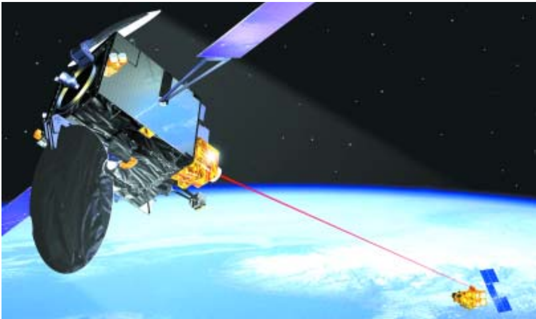
Artemis is designed to demonstrate new technologies such as mobile communications and inter-satellite laser links.
