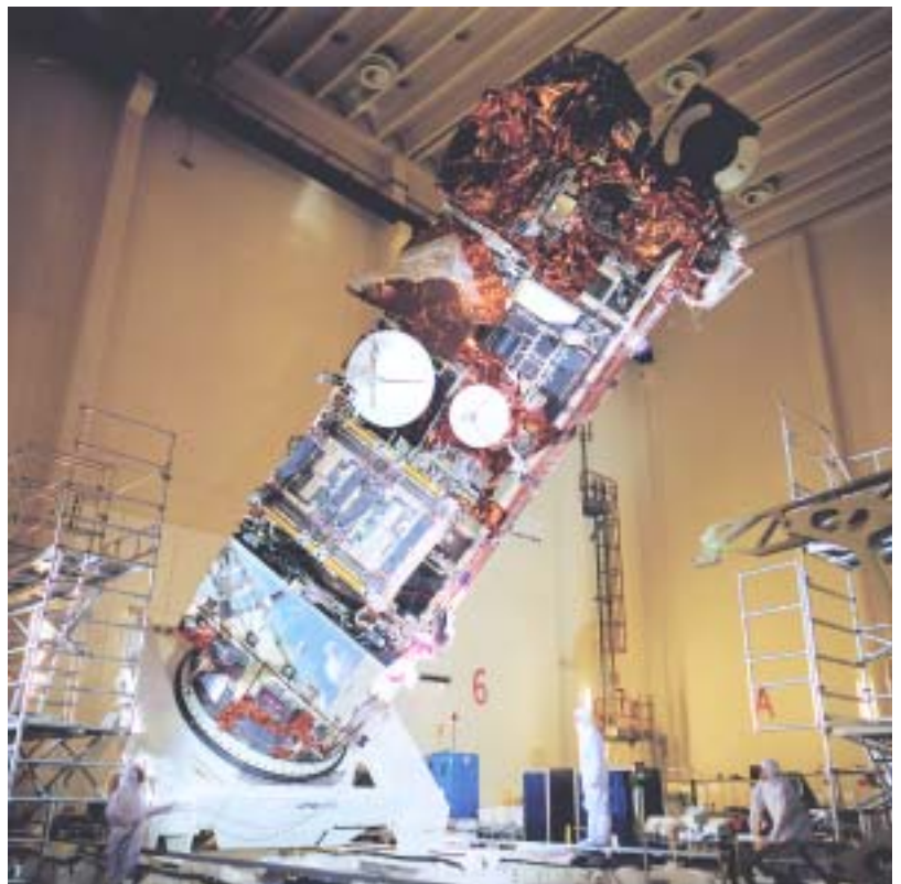
Envisat flight model during integration and alignment tests at ESTEC. (ESA)
