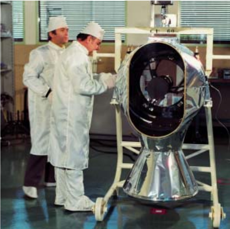
Meteosat's single Earth-observing instrument is the imaging radiometer.
