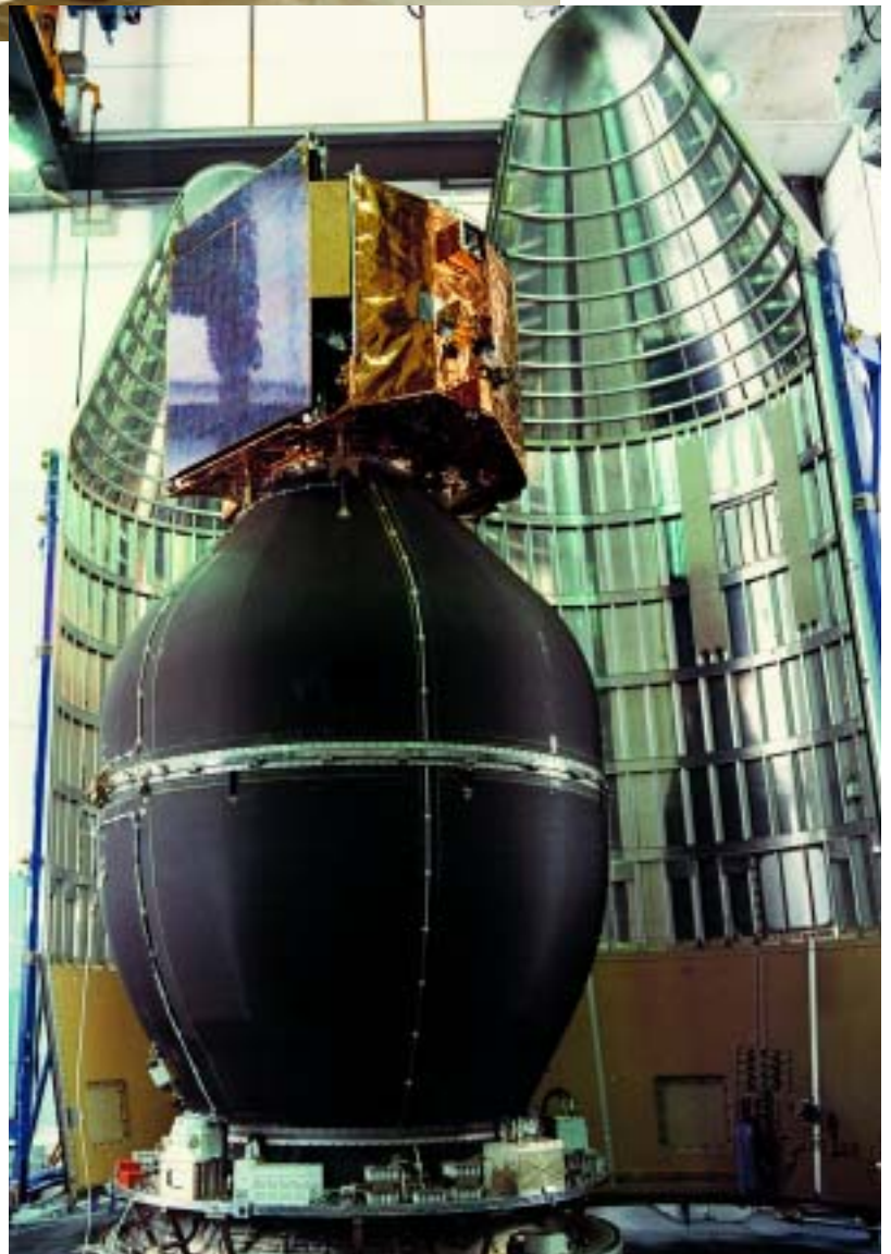
ECS-1 ready for launch. The black Sylda canister carried a second satellite. (CSG/Arianespace)
