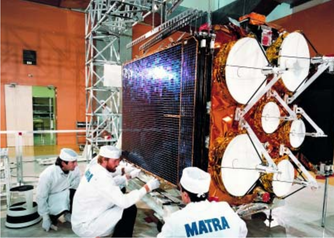
ECS-1 undergoing solar array deployment tests at Matra.
