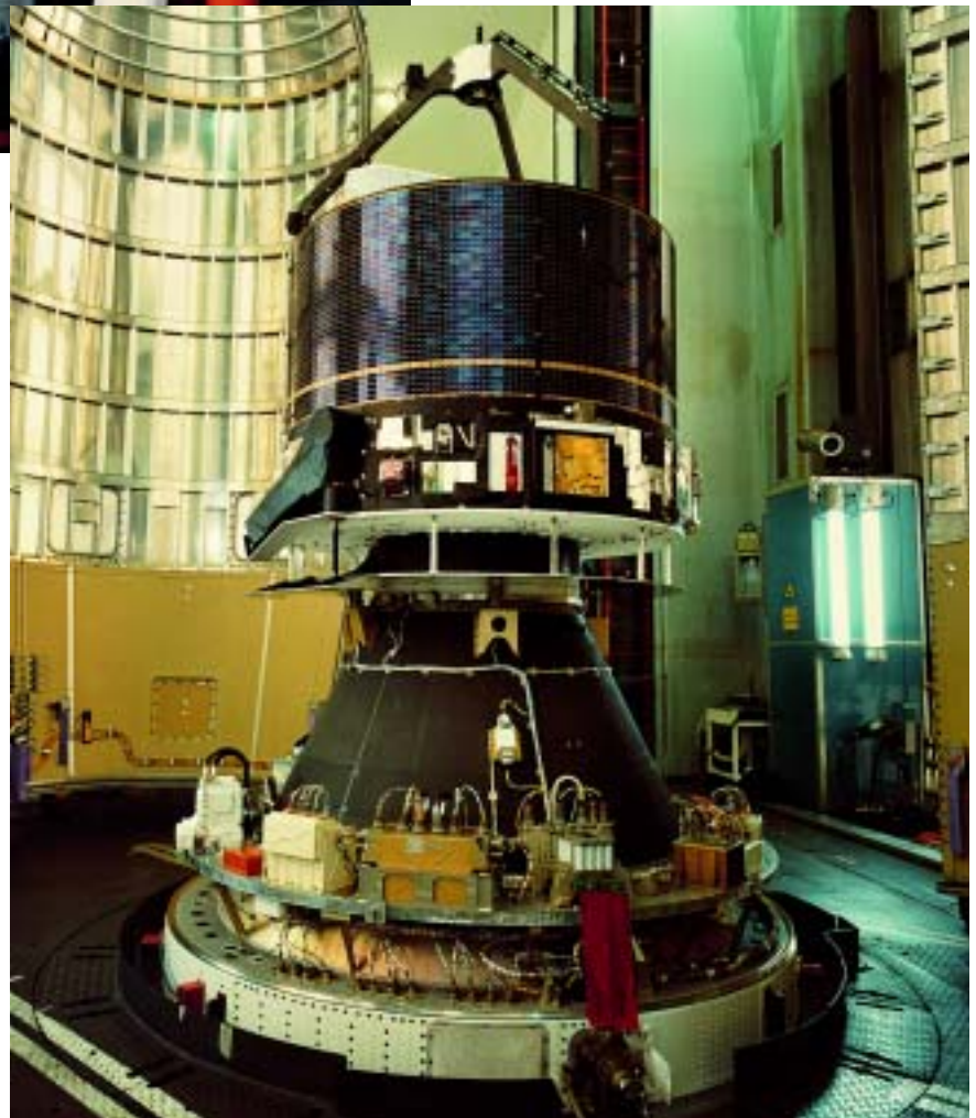
The Giotto Halley's Comet probe installed on top of its Ariane-1 launcher. The Vehicle Equipment Bay carries the rocket's control electronics. Behind, to the left is one half of the fairing. (ESA/CNES/CSG)
