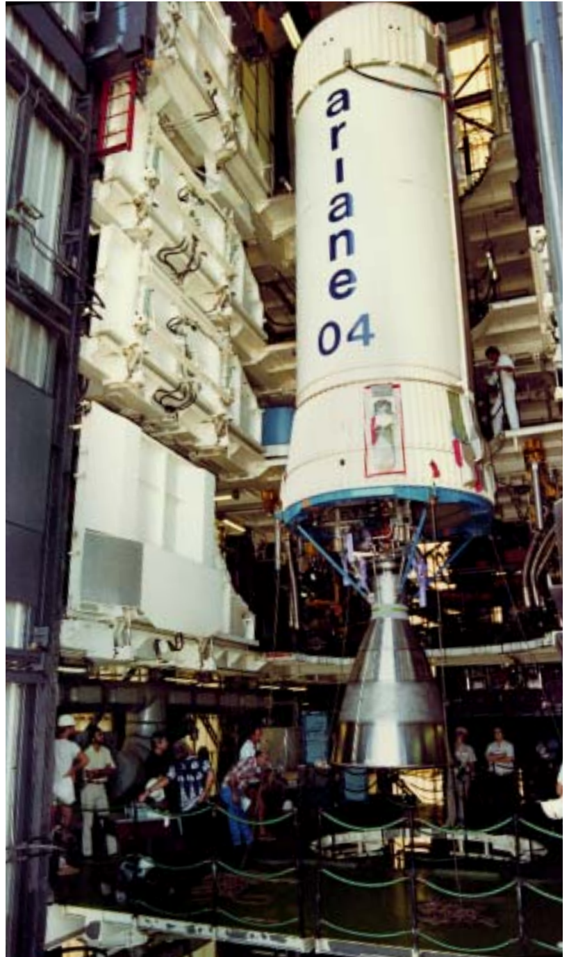
Stage-2 is powered by a single Viking engine. (ESA/CNES/CSG)
