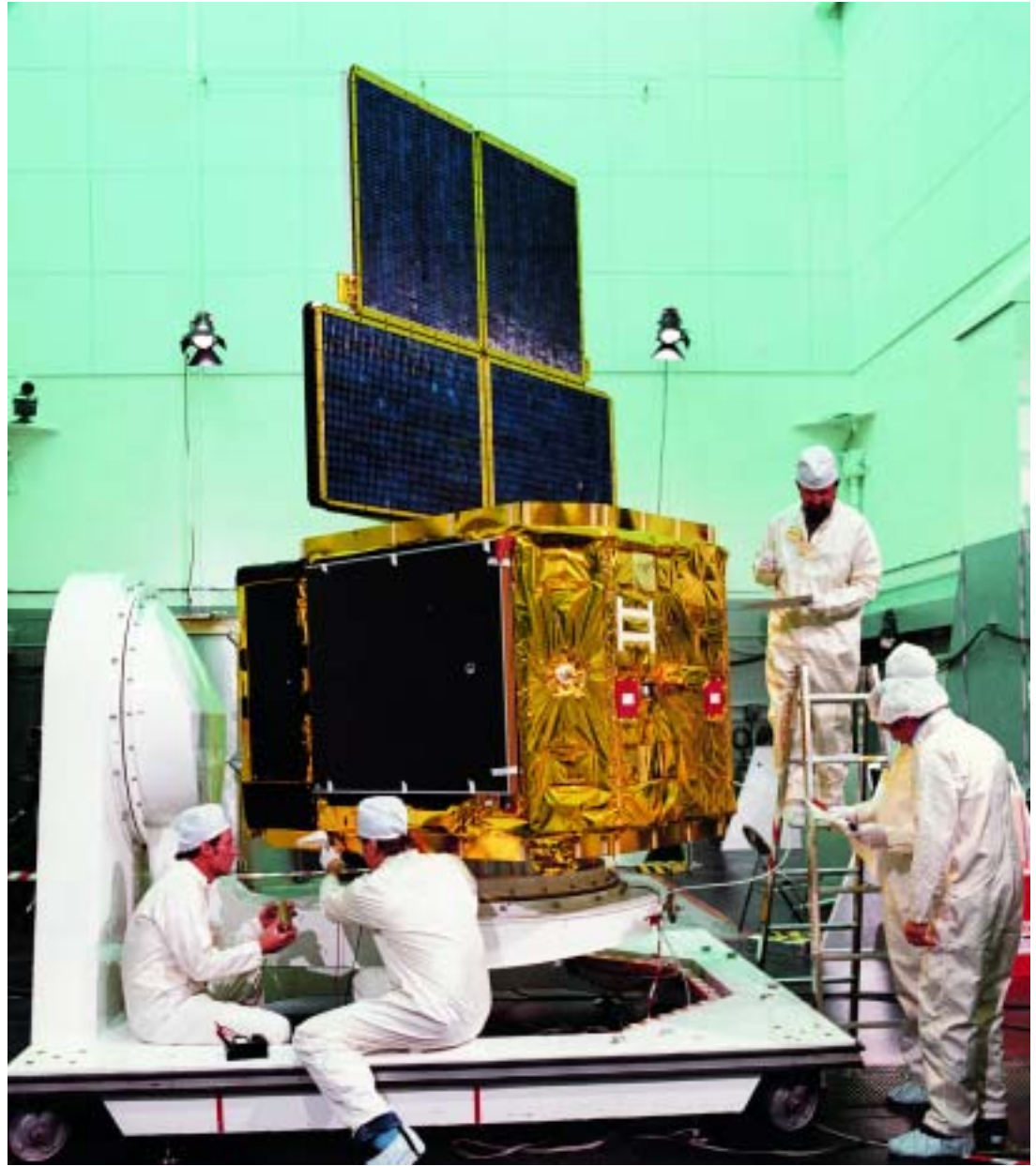
Exosat being prepared for launch from Vandenberg Air Force Base, California. The medium-energy and low-energy instruments are protected by their shutters on the left-hand face. These shutters were opened in orbit to act as sun shades for the telescopes.
