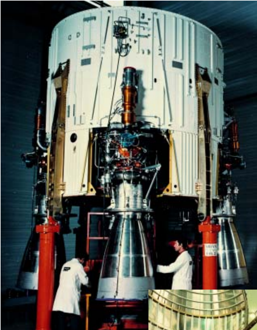
The engine bay of Ariane's first stage carries four Viking 5 engines. (Sneema Moteurs)
