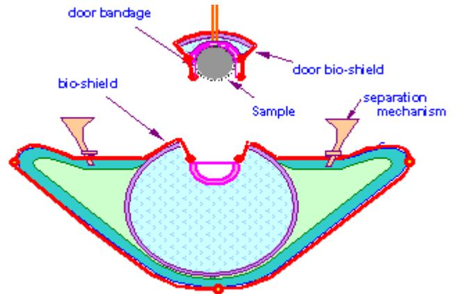
**Figure 6-1: EEV Contamination Protection and Sample Containment\***
