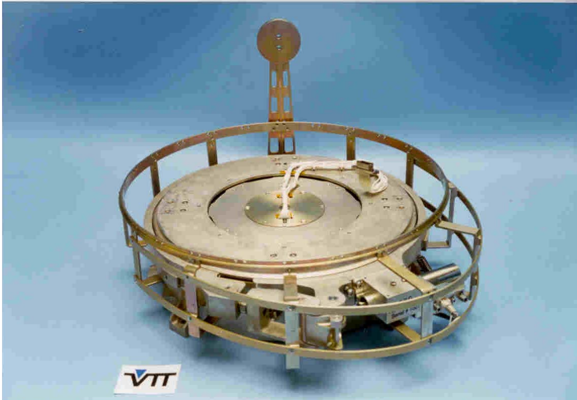
Figure 4.4.2: The rotating platform developed by VTT (Finland) for the MIMI instrument flown on Cassini.
