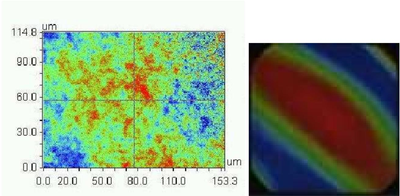
**Figure 1.** The surface roughness of high-grade commercial wafers is measured to be between 0.4 and 0.5 nm RMS between 5 and 500  $\text{mm}^{-1}$  (left, 5 nm peak to peak). An interferogram of a sliced wafer (right) shows that it is dominantly cylindrically curved, however by no more than 1.5  $\mu\text{m}$  peak to peak, corresponding to an image resolution of 1 arcsec.
