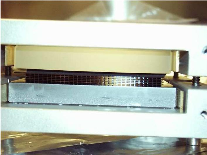
**Figure 6.** Front side of a prototype stack consisting of 6 plates of 70x70 mm<sup>2</sup>, providing 5x31 pores with a total area of 2 cm<sup>2</sup>.
