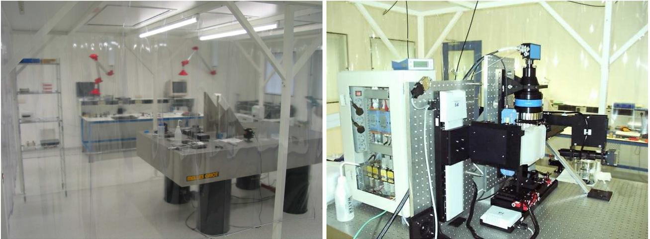
**Figure 4.** A fully automated stacking robot was developed to stack the plates. The setup is placed in a class-100 environment in the cosine clean room laboratories.
