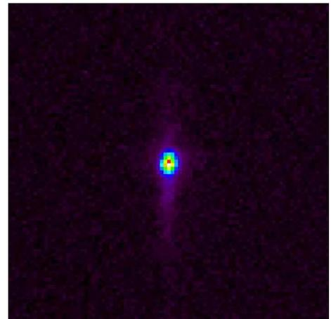
**Figure 7.** Measurements of the reflectivity and scattering confirm the excellent surface roughness of the wafers also after processing (left). The reflected spot with a footprint of 0.05x5 mm on the surface of the mirrors is not noticeably larger than the incident beam, which has a divergence of 1.5 arcsec (right).
