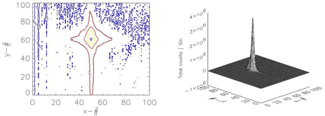
**Figure 8.** The point spread function of one of the measured stacks as constructed from pencil beam measurements over the central 70% of the aperture. The HEW is 5.3 arcsec. The FWHM of a single stack is 7.9 arcsec, which is large compared to the HEW due to the large asymmetry of the PSF.
