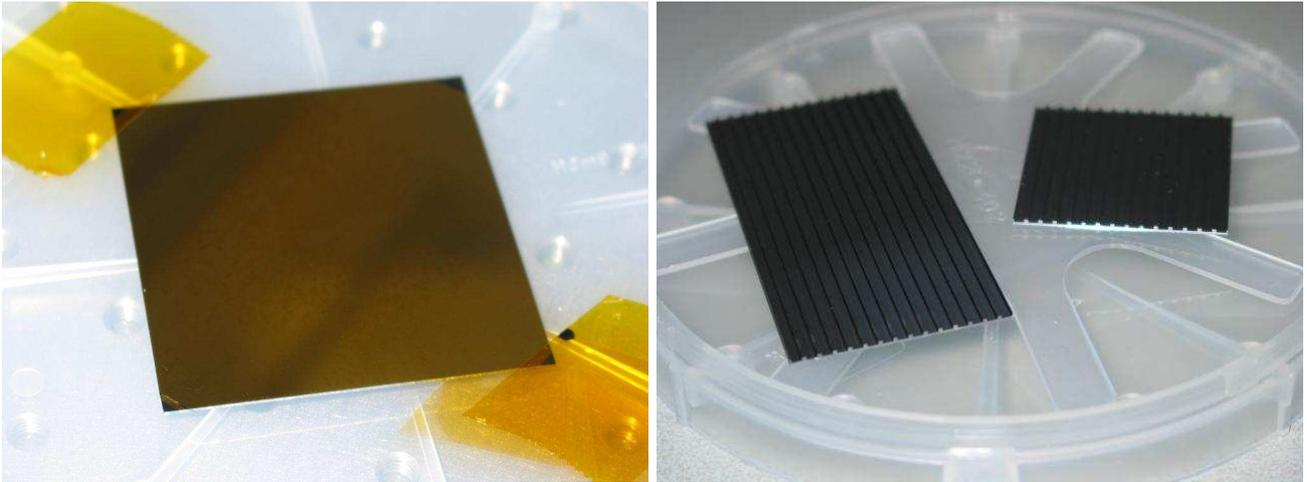
**Figure 2.** The optics are built up from rectangular cuts of commercial silicon wafers (left). The wafers are processed chemo-mechanically such that ribs remain, providing a thin membrane with ribs of very accurate height and highly polished surfaces (right).
