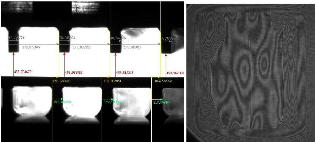
**Figure 5.** Real-time image analysis of digital microscope images provides alignment to  $\mu\text{m}$  accuracy (left). Interferometry is used to measure the shape of the plates to high accuracy during stacking (right).
