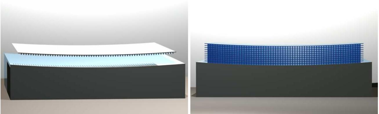
**Figure 3.** Ribbed plates are stacked onto a mandrel that provides the correct starting curvature.
