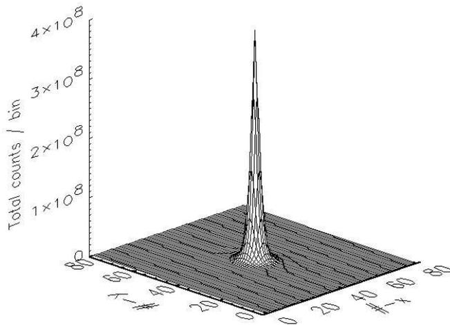
**Figure 9.** The point spread function of one of the measured stacks, taking into account the effect of placing the stacks along a full circle just as it would be in the final optic. The encircled energy is again 5.3 arcsec, but the FWHM is reduced to 3.1 arcsec.
