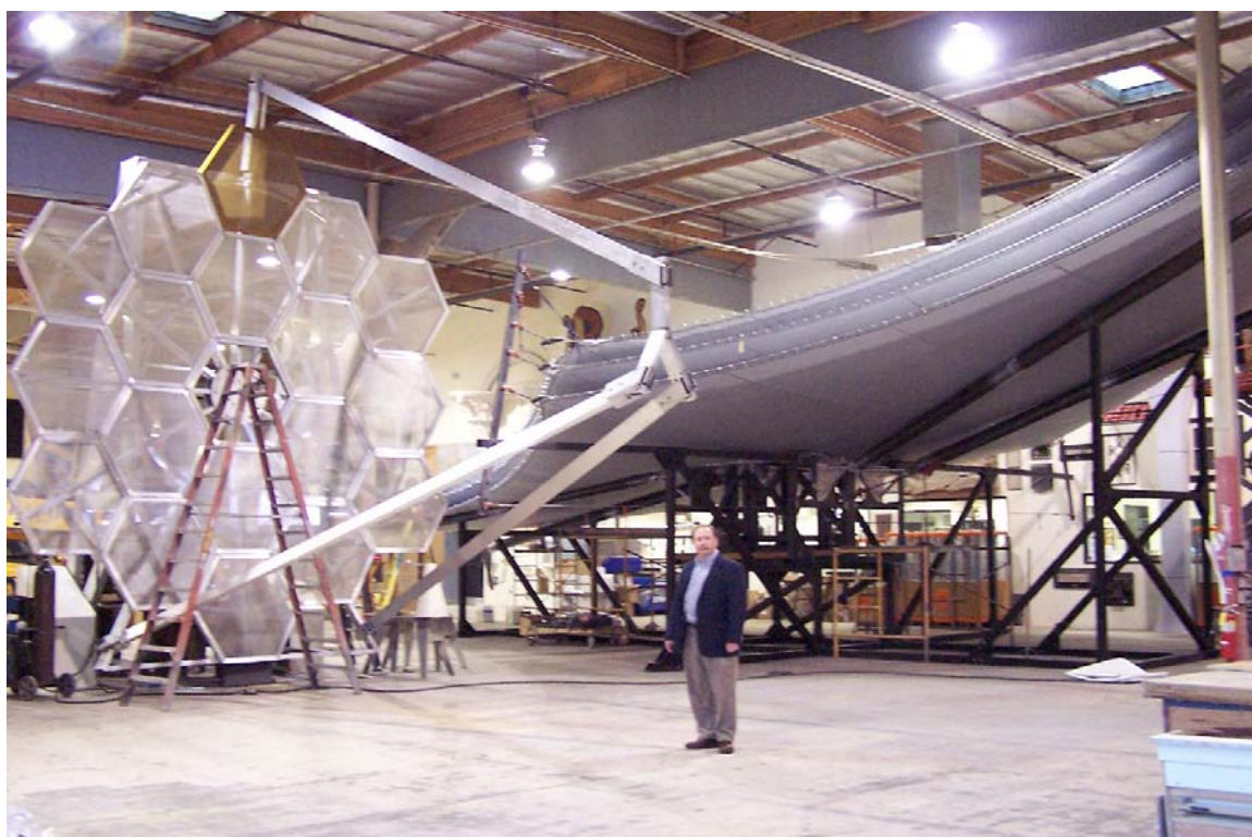
Full scale mock-up of the deployed 18-segment JWST telescope at the US prime contractor. To the right is a matching mockup of the deployed Sun Shield (Northrop-Grumman Space Technology).
