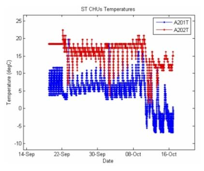
ST CCD Temperatures (A201T= CCD1; A202T=CCD2)
