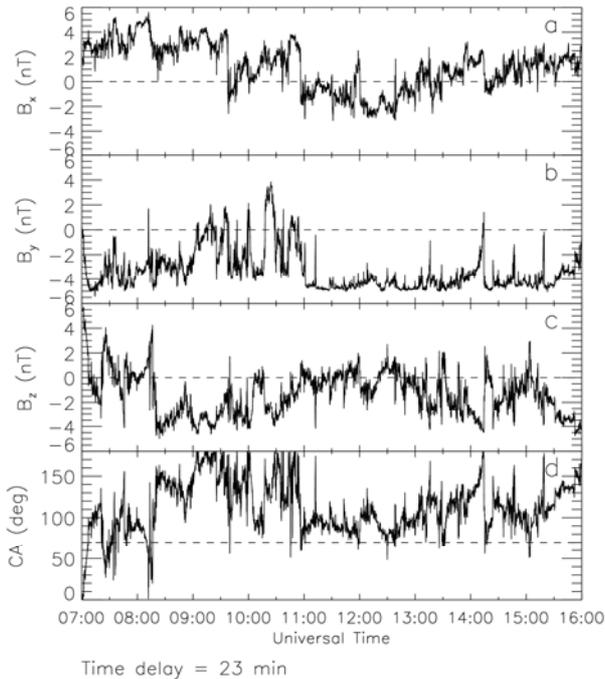
Fig. 2. Wind IMF data in GSM coordinates, lagged with 23 min, for the period 07:00-16:00 UT. Panels (a), (b), (c) show the  $B_x$ ,  $B_y$  and  $B_z$  components of the IMF and panel (d) shows the IMF clock-angle.
