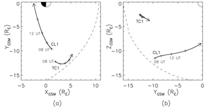
Fig. 1. Trajectories of Cluster/sc1 and TC-1 for the period 08:00-16:00 UT, in GSM coordinates. (a) in the  $XY$  plane, (b) in the  $YZ$  plane. Black crosses along the orbits are separated by 2 hours. A model of the magnetopause position (see text for details) is indicated in the  $Z_{GSM} = 0$  plane (panel a) and in the  $X_{GSM} = 0$  plane (panel b) by the dashed line.
