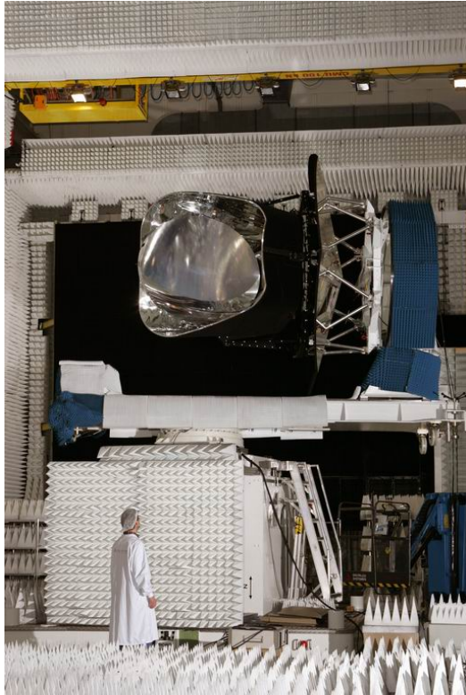
(left) The Radio Frequency Qualification Model of Planck being tested in the CATR at Alcatel; and (right) the PFM1 model before shipment to the Centre Spatial de Liège.
