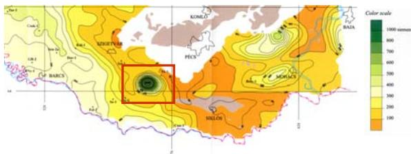
Fig. 1. The telluric conductivity anomaly at MagyarMEcske, Hungary, on the Telluric Conductance Map of Transdanubia ([2])
