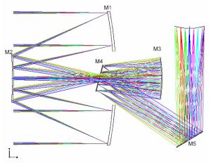
Figure 3 Telescope optical design for WFI
