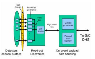
Figure 4 Block-diagram of the WFI camera
