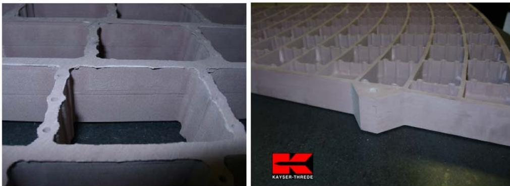
Figure 10 Sintered CeSiC prototype optical petal demonstration unit. Images courtesy of Kayser Threde
