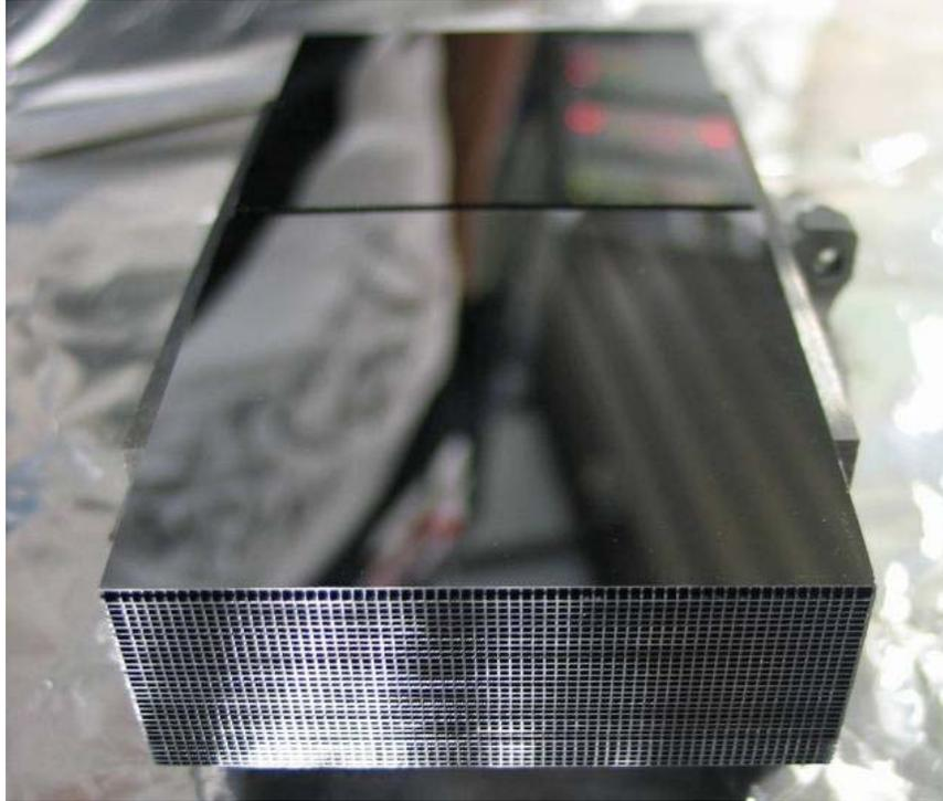
Figure 9 Second completed XOU tandem, now integrated into a low mass CeSiC bracket representative for flight-like design
