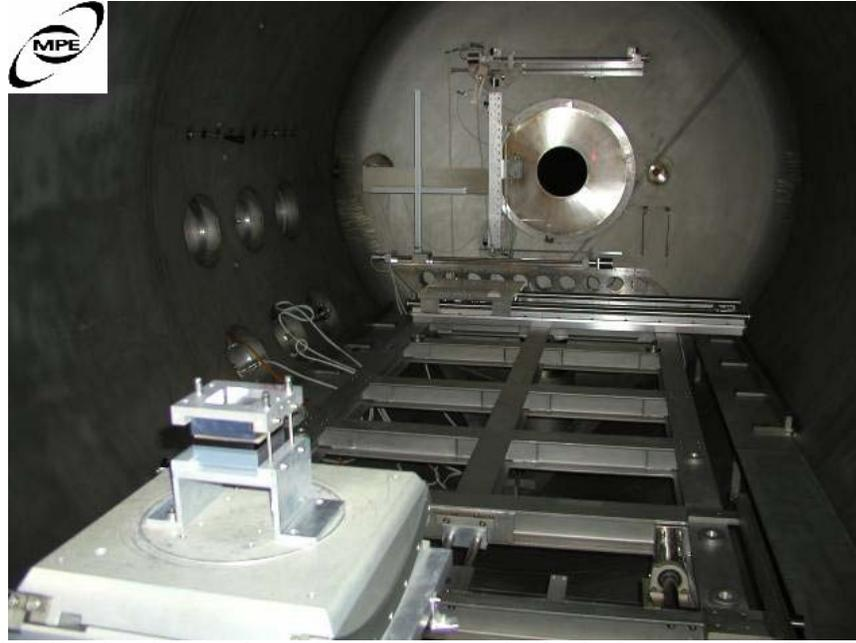
Figure 22 HPO stack module placed inside Max Planck Panter chamber for the purpose of checking interfaces for future full beam illumination tests. Image courtesy MPE.
