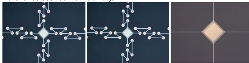
Figure 21 – Various prototype ESI detectors tested at SRON. The detector on the right demonstrated close to the goal performance.
