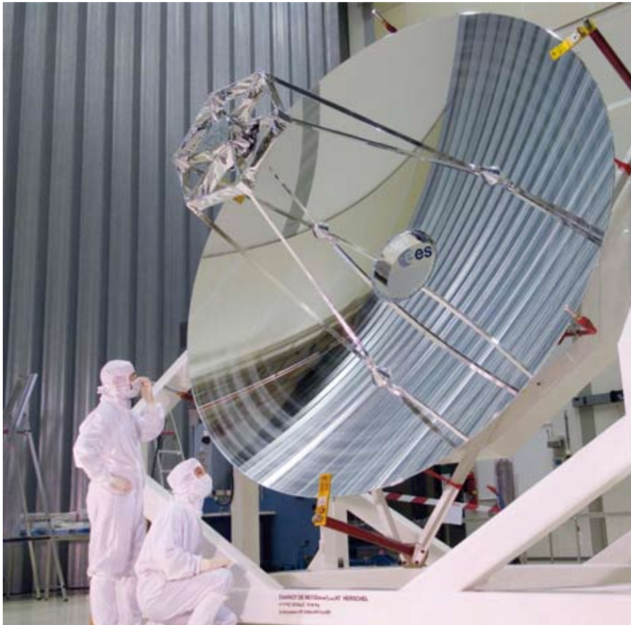
Figure 4.2.2. The Herschel flight telescope during incoming inspection in the ESTEC Test Centre in late Jan 2008. (ESA)
