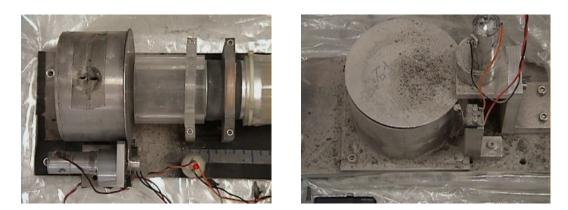
Projectile deeply embedded in the regolith simulants
