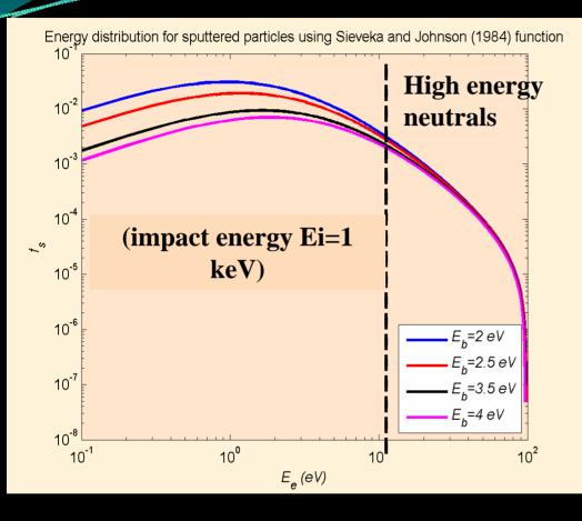
where  $E_e$  is the energy of the ejected particle,  $E_i$  is the energy of the incident particle and  $E_b$ is the binding energy
