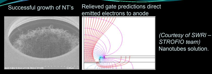
As power resources on spacecrafts are usually very limited, different approaches to the conventional hot filament to generate the electrons needed for the electron impact ionization process, have been investigated. The yield and linearity of the source and the lifetime characteristics can be experimentally investigated.
