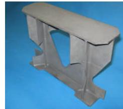
Figure 4-1 pictures from manufactured representative ribs: 1.5mm thick, 200mmheight. Skin thickness is 3.8mm. These ribs demonstrate the capability to manufacture the mirror stiffeners.
