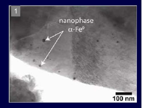
1) TEM image of NWA 2737 olivine. Small, dark (electron-dense) spherules are consistent with  $\alpha$ -iron kamacite [after Treiman *et al.*, 2007] (Pieters *et al.*, 2008)
