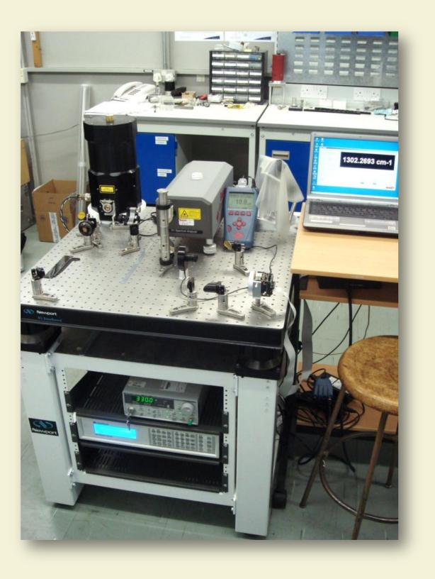
7.7 μm QCL mounted on a substrate and installed in a custom made laser head
