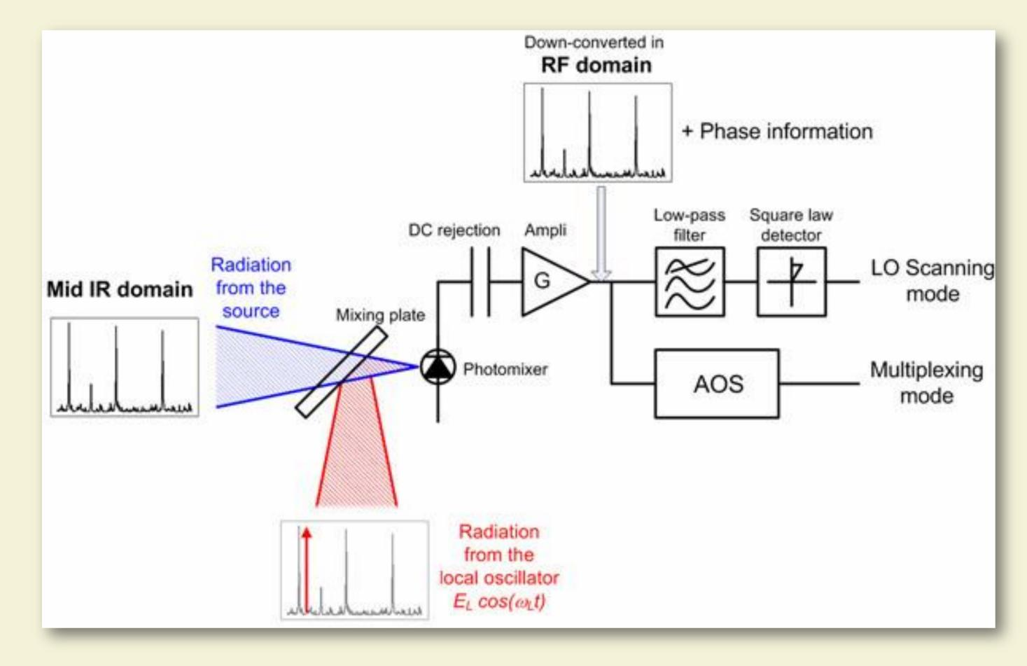
Schematic of the prototype LHR instrument
