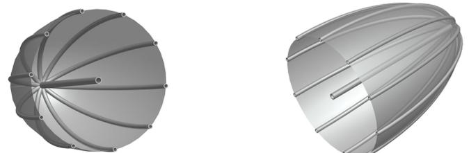
**THE INFLATABLE APPROACH:** The entire envelope will be fabricated on Earth as a single piece and flexible fiber tube joints to allow packing. Upon landing on the Mars' surface the envelope would be pressurized and epoxy resins rapidly pumped into the tubes to solidify and thus forming a rigid structure and then the vacuum pump takes over.
