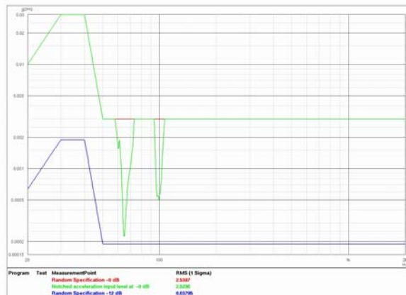
Fig. 9. Comparison of qualification notched limit level to low level run input in X axis
