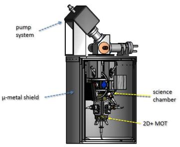
Figure 16: Sounding rocket design of the Physics Package
