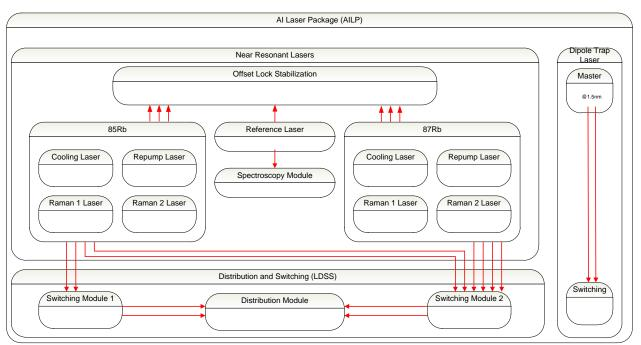
Figure 18: Example Block Diagram of AI Laser Package (redundant lasers are no shown)
