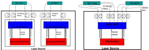
Figure 7: Preliminary Design of STE-QUEST Atomic Clock Laser Source: baseline design based on Pharao heritage (left) and alternative design based on telecom fibre lasers (right)
