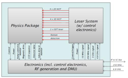
Figure 14: Atom Interferometer Top-Level Block Diagram
