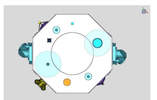
Figure 23: Placement of the two LCT heads on the CDF model of STE-QUEST. Placement on two different, opposite panels ensures the common view capabilities.
