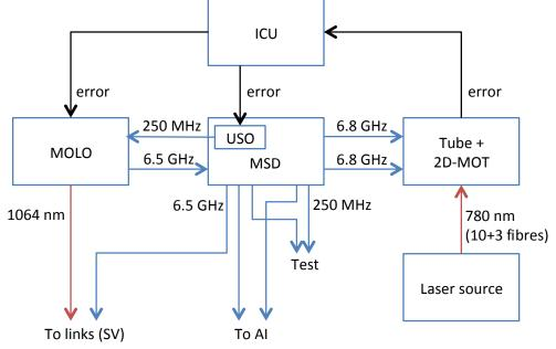
Figure 4: Clock Subsystem Block Diagram
