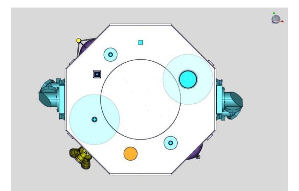
Figure 21: Antennae placement from the CDF study (light green shades denote minimum obstruction-free zones) .
