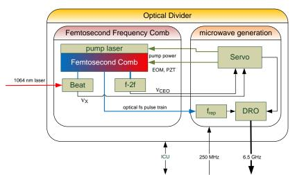
Figure 11: Block Diagram of MOLO Optical Frequency Divider
