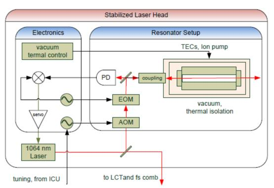
Figure 9: Block Diagram of MOLO Stabilised Laser Head
