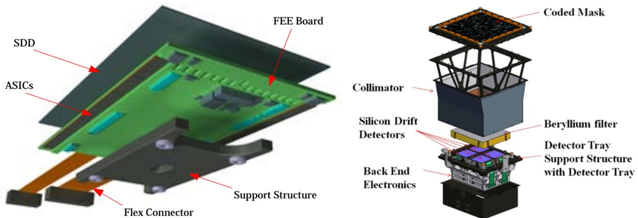
Figure 10: LAD Detector Assembly (left) comprising Silicon Drift Detector (SDD), and Front End Electronics (FEE) Board with readout ASICs; WFM Design (right)
