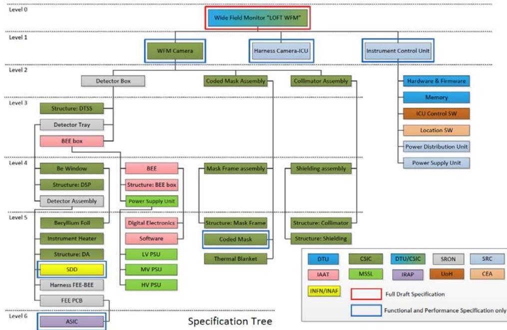
Figure 4: WFM specification tree, indicating those specifications provided at I-PRR (blue/red outlines)
