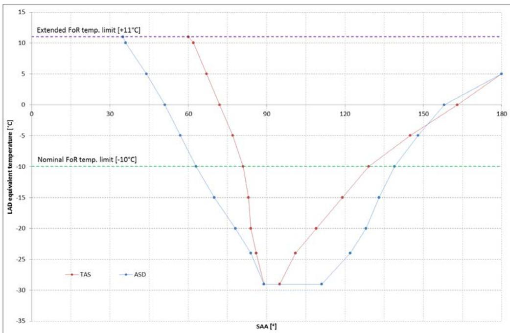
Figure 7: TAS and ASTRIUM SC orbital average (not taking into account  $\sim\pm 5$  deg C variation along the orbit) predicted LAD equivalent temperature as a function of Sun aspect Angle
