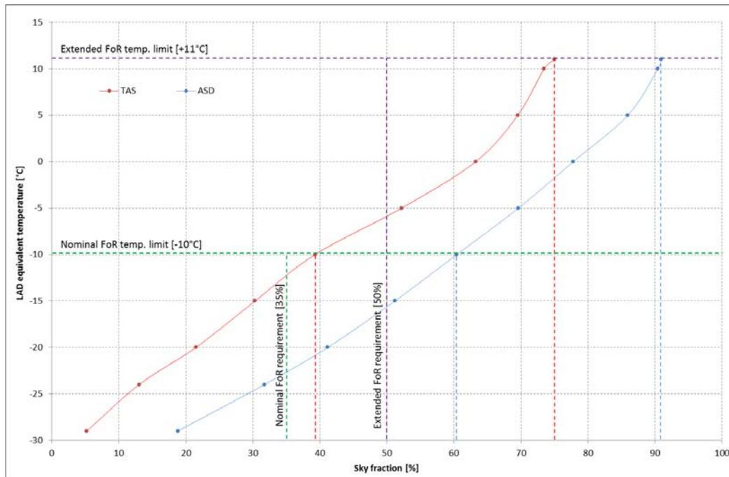
Figure 8: TAS and ASTRIUM SC orbital average (not taking into account +/-5deg C variation along the orbit) predicted LAD equivalent temperature as a function of Sky Visibility
