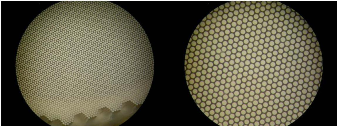
**Figure 11: Magnified photographs of the small-size, 100  $\mu\text{m}$  pore capillary plate produced by Hamamatsu (Japan) to test the feasibility of the LOFT specifications**
