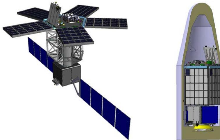
Figure 6: TAS-I SC design (also shown stowed in fairing)
