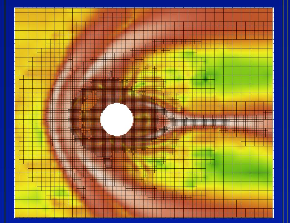
2-D cut of an MHD simulation of the plasma density around the Earth generated by the GUMICS-4 code (see Janhunen et al. 2012)
