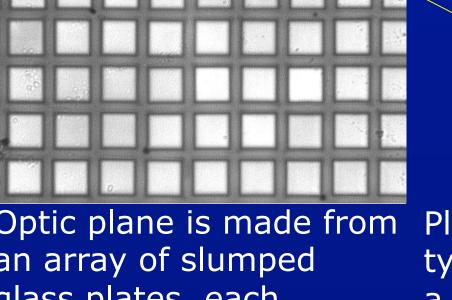
an array of slumped glass plates, each typically 4 cm x 4 cm, of 1 mm thickness.
