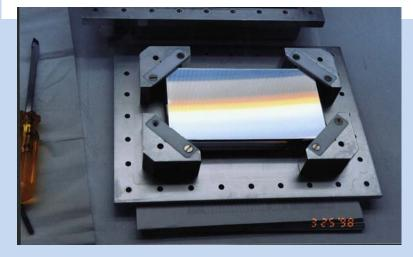
Ion etched, blazed grating. MoSi multilayers for high reflection Spherical figure, 2.2m focal length
