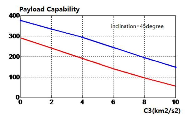
Escape from a 200 x 900 km parking orbit (blue curve) and a 200 km circular parking orbit (red curve)
