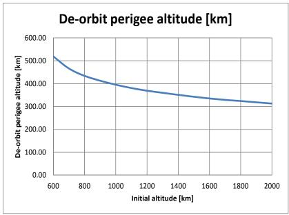
Required perigee as a function of initial apogee altitude for eccentric de-orbiting solution (corresponds to the blue curve in the left figure)
