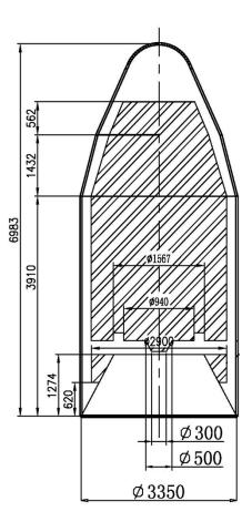
LM-2D fairing static envelope with 1194 (left) and 937 (right) interfaces
