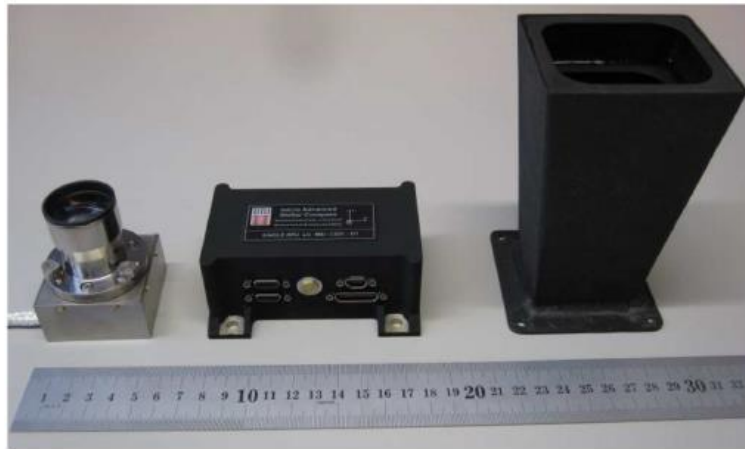
Figure 9-9: DTU \mu ASC star tracker (left: CHU - Camera Head Unit, middle: DPU – Digital Processing Unit, right: baffle)
