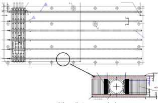
All radiator panels have embedded heat pipes
