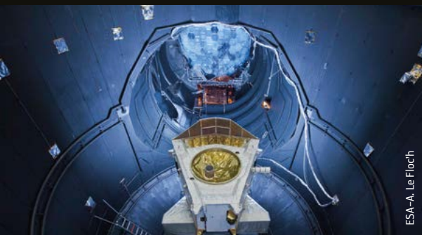
The MTM Structural and Thermal Model in the Large Space Simulator, ahead of a 12-day Sun-simulation test
