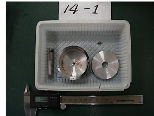
Target and Projectile (left) and Conical Horn and Catcher (right) after the Capsule Recovery
