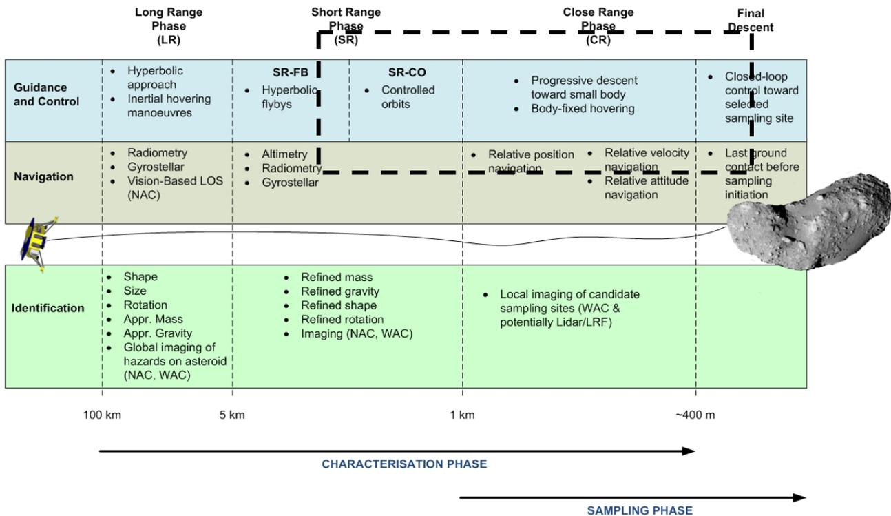
**Figure 7.1-1: Characterization and Sampling Phases**
