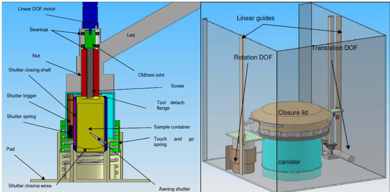
Figure 6.1-1 Overview of the sampling tool (left) and Transfer system with 2 DOFs (right)
