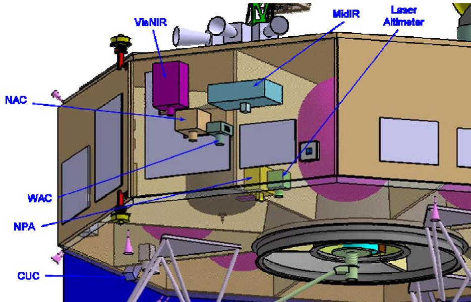
**Figure 2.2-2 Payload Accommodation on the Spacecraft**
