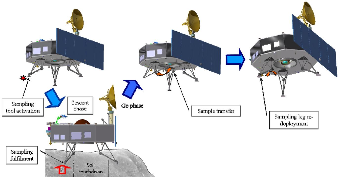
**Figure 5.2-1: Operational sequence for the sampling collection**
