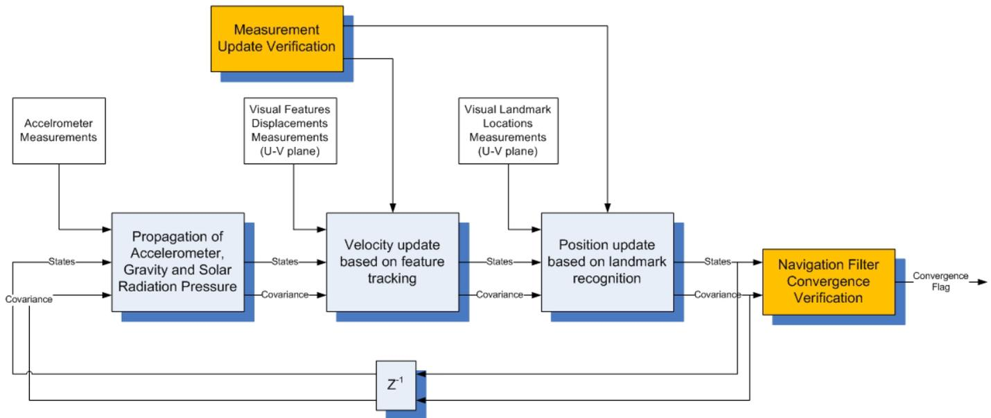
**Figure 7.2-1: Block Diagram of Translational State Estimator**
