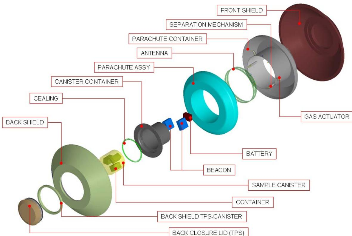
**Figure 8.1-1 ERC Exploded View – Main Components**
