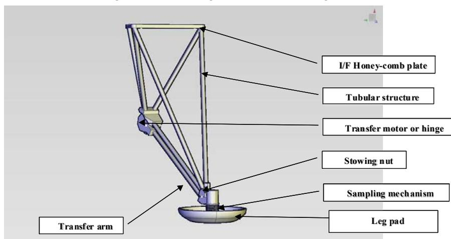
**Figure 5.1-1 T&G motorized legs in deployed configuration**
