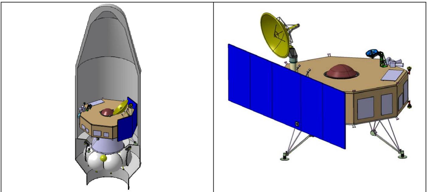
**Figure 2.2-1 Marco Polo Spacecraft Stowed/Deployed**
