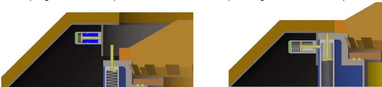
**Figure 8.2-1 Parachute Deploy Mechanism Locked (Left) and released (Right) Configuration**
