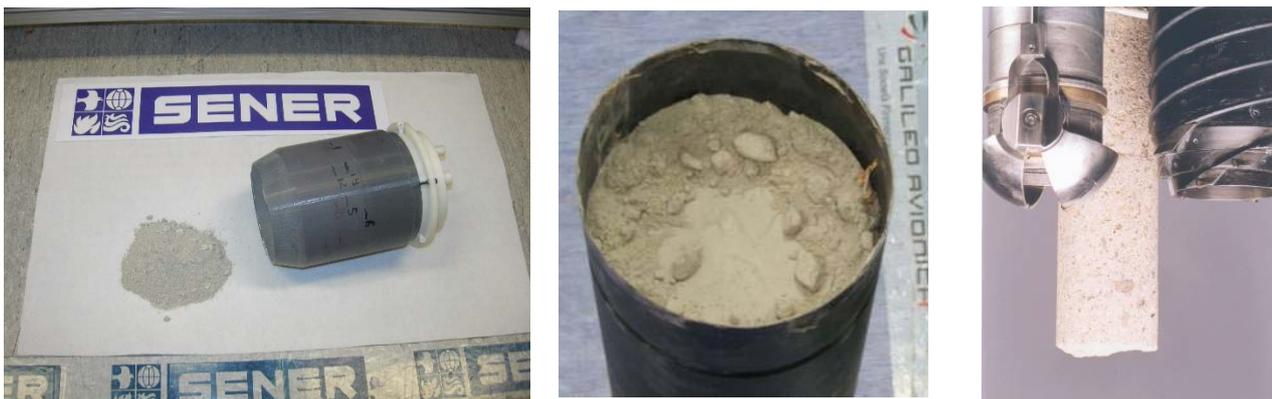
Figure 33: Sample simulant material collected in various tests based on the coring method. Fine powder mixed with cm-sized fragments on the left and in the centre, and hard core on the right.
