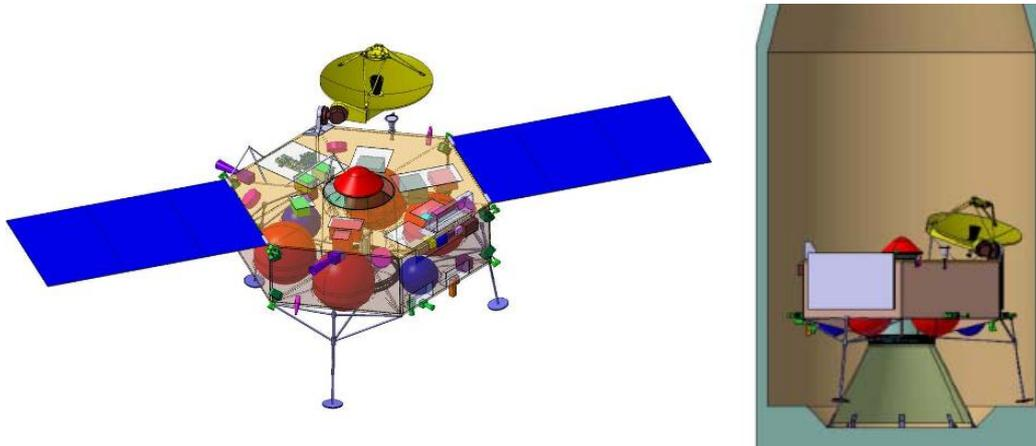
Figure 41: Spacecraft design option A configuration of main spacecraft
