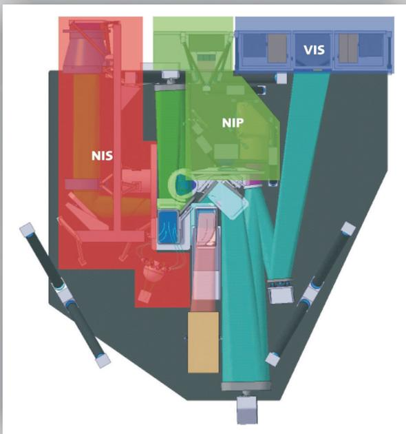
The instruments are realized as individual entities with the defined interfaces to the payload module. Each instrument has its own base plate. The radiators are aligned on the cold side of the spacecraft.
