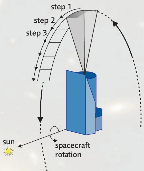
The sky is nominally observed along great circles in planes perpendicular to the Sun-spacecraft axis (SAA=0). The advantage is optimum thermal stability. The drawback of temporal inefficiency is solved by observing also during the dead times around the Equinoxes. The required spacecraft tilt away from the sun results in solar aspect angles SAA>0.
