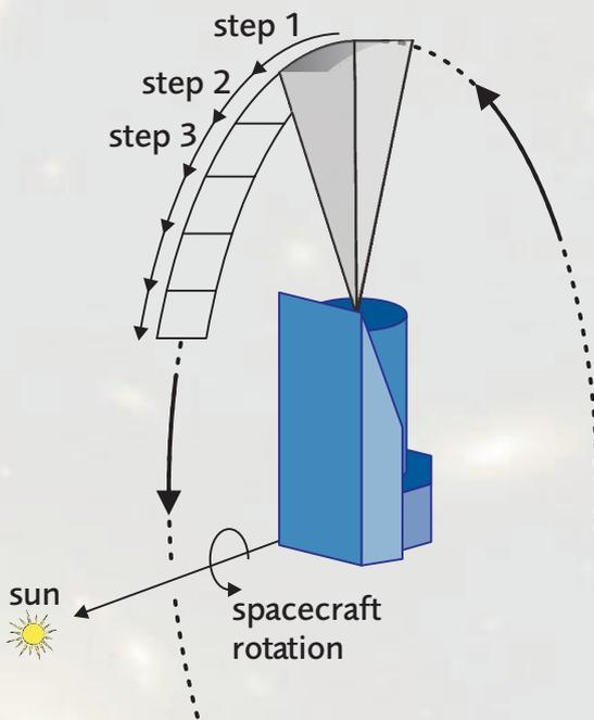
The sky is nominally observed along great circles in planes perpendicular to the Sun-spacecraft axis ( $SAA=0$ ). The advantage is optimum thermal stability. The drawback of temporal inefficiency is solved by observing also during the dead times around the Equinoxes. The required spacecraft tilt away from the sun results in solar aspect angles  $SAA > 0$ .
