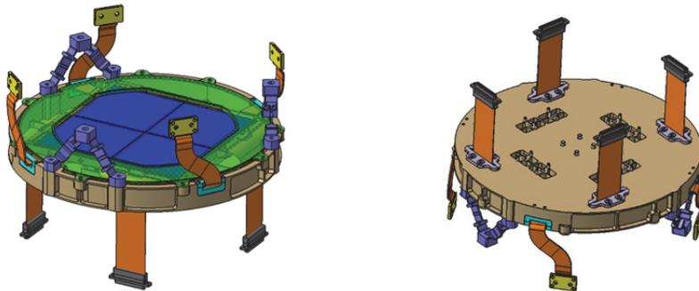
Figure 4.6: The Focal Plane Assembly seen from top (left) and from bottom (right). In blue the array of 4 CCDs and in green the straylight mask. FPA is supported by 3 bipods to the TOU structure. 3 thermal straps evacuate the heat. Each CCD is connected by a flexi to the FEE box.
