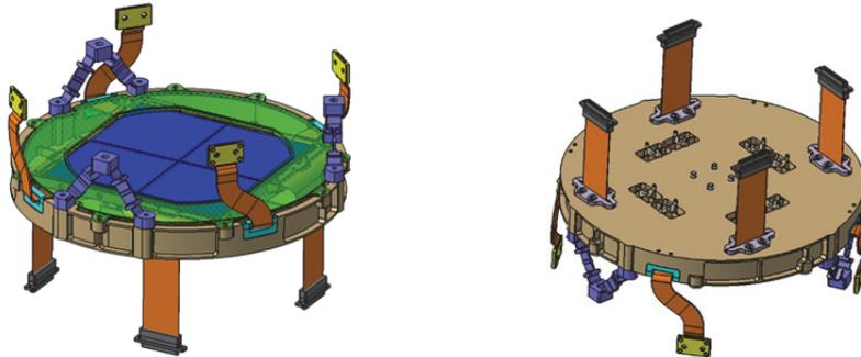
Figure 4.6: The Focal Plane Assembly seen from top (left) and from bottom (right). In blue the array of 4 CCDs and in green the straylight mask. FPA is supported by 3 bipods to the TOU structure. 3 thermal straps evacuate the heat. Each CCD is connected by a flexi to the FEE box.
