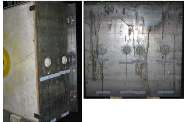
Fig. 9. Right: side of the target block, showing the steel casing and two of the integrated pressure gauges; Left: rear side of the target with 4 gauges integrated
