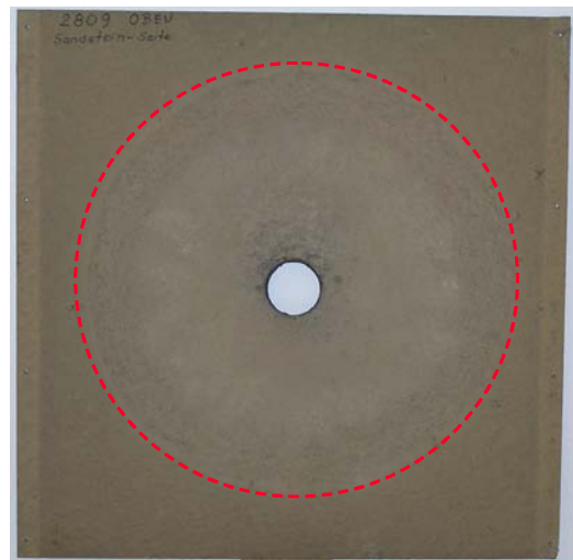
Fig. 12. Damage from uprange ejecta in fragment catcher in Exp. 2809 (wet sandstone)
