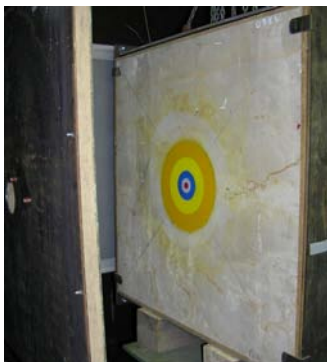
Fig. 8. Target set-up: left: fragment catcher, right: sandstone block
