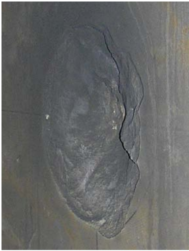
Fig. 10. Impact crater in wet sandstone - perspective
