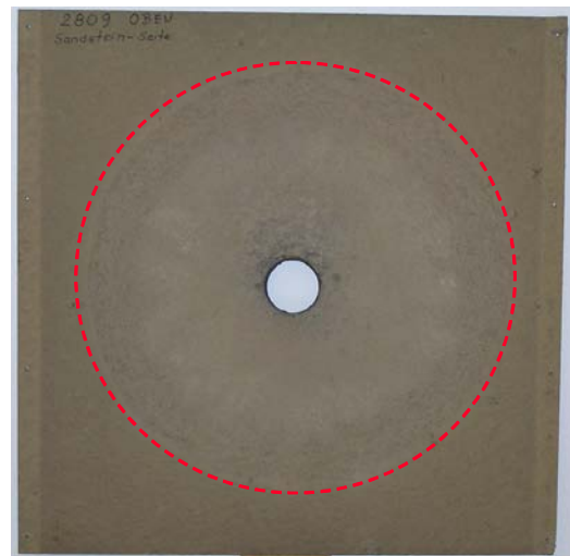
Fig. 12. Damage from uprange ejecta in fragment catcher in Exp. 2809 (wet sandstone)
