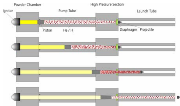
Fig. 5. Working principle of a two-stage light-gas gun
