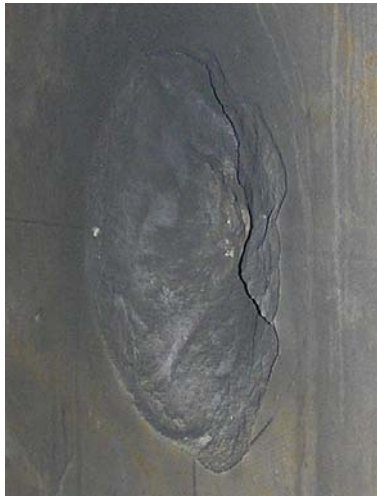
Fig. 10. Impact crater in wet sandstone - perspective
