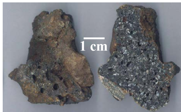
Fig. 3. Thermally altered cobble, cut in slices, pumice-like structure with signs of volatilisation
