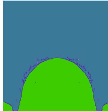
Fig 8 – Crater formation using GRIM for Coesite 10ms after impact
