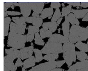
Fig. 3. Microscopic picture of target material, showing sand particles and voids (black)
