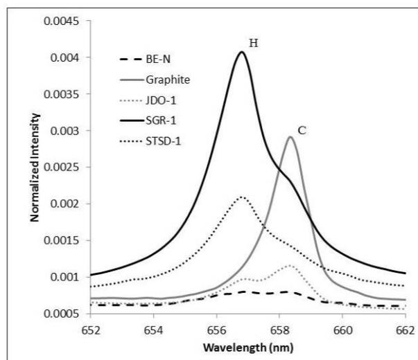
Figure 1. H (656.5 nm) and C (658.8 nm) peaks in geochemical reference standards; BE-N (basalt, 2000 ppm C), Graphite (99.9 wt% C), JDO-1 (dolomite, 12.8 wt% C, 0.17 wt% H<sub>2</sub>O), SGR-1 (petroleum shale, 28 wt% C), STSD-1 (stream sediment, 12.3 wt% C, 4.5 wt% H<sub>2</sub>O). Intensity has been normalized to the total emission for each spectral range.
