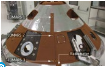
COMARS+ sensors on Schiaparelli http://exploration.esa.int/mars/57377
