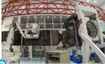
Deployment test of the Trace Gas Orbiter solar arrays http://exploration.esa.int/mars/56917
