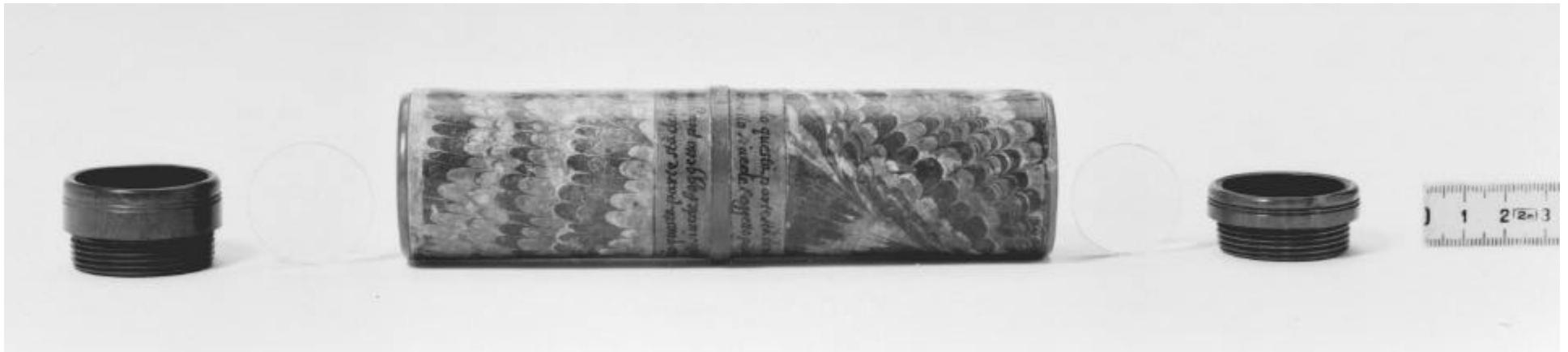
The erector is mechanically symmetrical but optically asymmetrical. Near the middle of the tube there is a cardboboard ferrule that fixes the position of the erector within the smallest draw tube of the telescope. On either side next to this ferrule is an inscription in ink. One side reads "When this part is inside the tube the object is seen larger"; the other side reads "When this part is inside the tube the object is seen more brightly".
