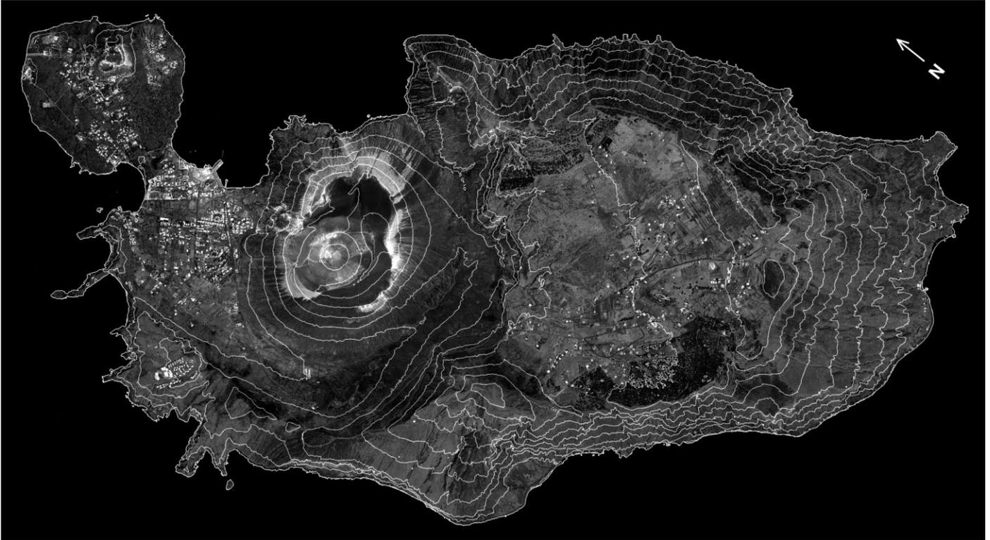
**Fig. 3.** HRSC orthoimage mosaic of Vulcano Island (I) with 50 m contour lines derived from HRSC stereo data. Obtained during the HRSC flight campaign of May 1997 at an altitude of 5000 m with a spatial resolution of 20 cm px<sup>-1</sup> for the nadir and 40 cm px<sup>-1</sup> for the stereo lines.
