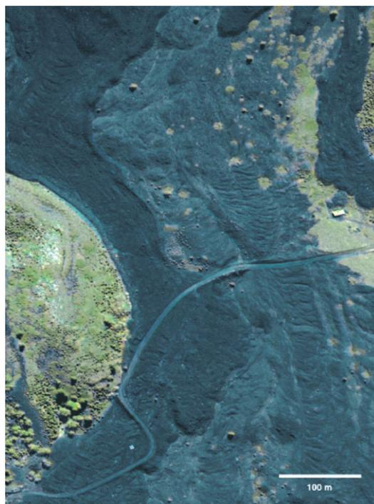
Fig. 14. HRSC test image of Mount Etna lava flows from a flight altitude of 10 km. Resolution is 40 cm px<sup>-1</sup>.
