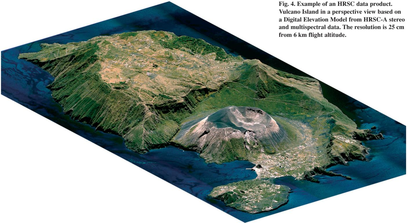
**Fig. 4.** Example of an HRSC data product. Vulcano Island in a perspective view based on a Digital Elevation Model from HRSC-A stereo and multispectral data. The resolution is 25 cm from 6 km flight altitude.
