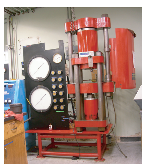
High pressure apparatus: Boyd-England-style piston cylinder
