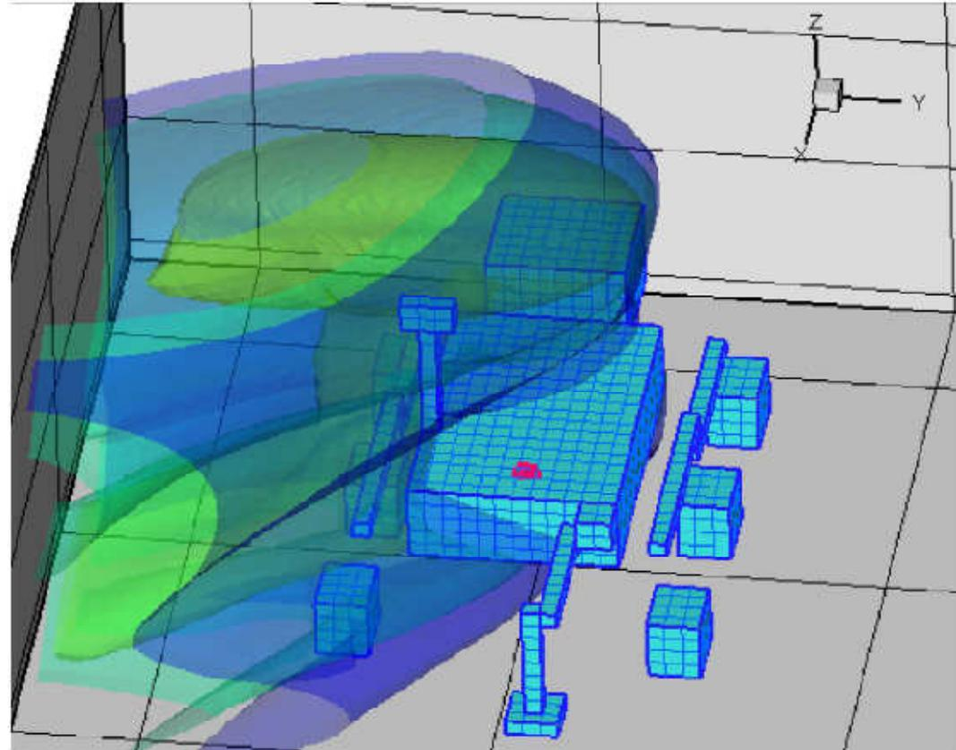
Results of an example calculation showing surfaces of 100 ppb, 10 ppb, and 1 ppb density for a contaminant emanating from a vent, not shown, located at the right rear of the rover body. The outermost contour corresponds to 1 ppb, the innermost contour to 100 ppb.
