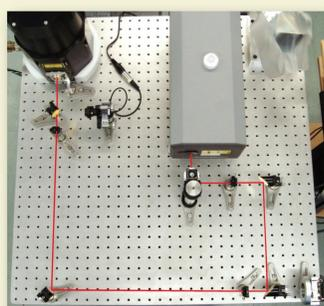
Setup of the optical bench during testing of the 7.7 μm QCL at the Rutherford Appleton Laboratory
