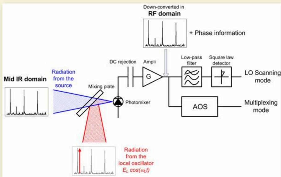
Schematic of the prototype LHR instrument
