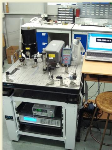
The design of the LHR allows for a compact and lightweight (approx. 5 - 10 kg) instrument. The current Quantum Cascade Laser based LHR at the Rutherford Appleton Laboratory has a dimension of 0.75 m x 0.75 m and there is potential for significant miniaturization through optical integration. It has also been shown that a carefully selected specific high resolution microwindow provides as much information as a medium resolution radiometer covering a broad spectral range<sup>[5]</sup>.
