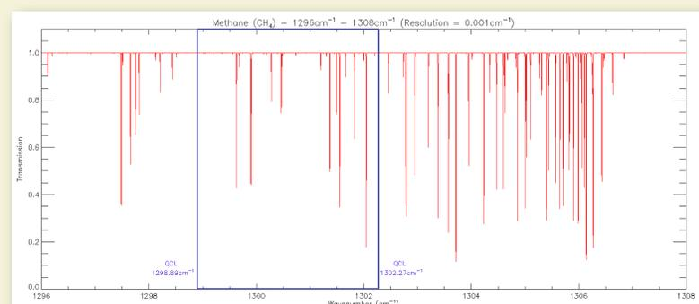
High resolution (0.001 cm<sup>-1</sup>) simulated CH<sub>4</sub> spectrum from 1296 - 1308 cm<sup>-1</sup> with the 7.7 μm QCL tuning range shown in blue
