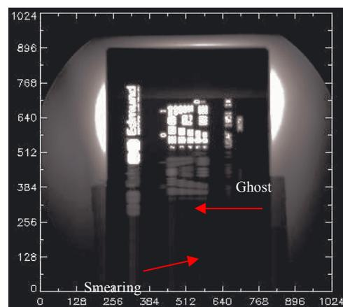
Figure 3 : Picture of the USAF target. Light intensity multiplied by 5 to show ghost and smearing.
