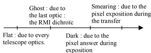
Figure 4 : Apparition of the defects in the image creation process.
