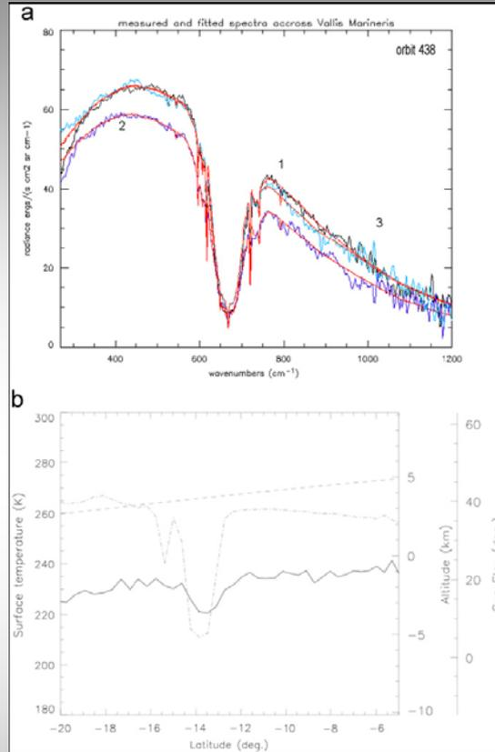
**Fig. 2.** (a) PFS measured spectra inside (2), on the edge of (3) and outside (1) Valles Marineris. Spectrum 2 shows lower temperatures and the water ice band at 750–900 cm<sup>-1</sup>.
