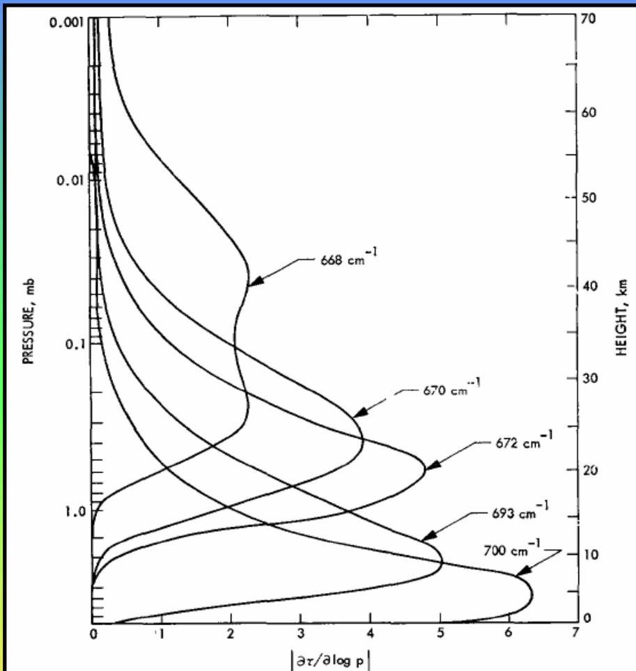
Sample weighting functions for the  $667\text{ cm}^{-1}$   $\text{CO}_2$  band. The examples shown give an indication of the height range over which information on the temperature profile can be obtained.
