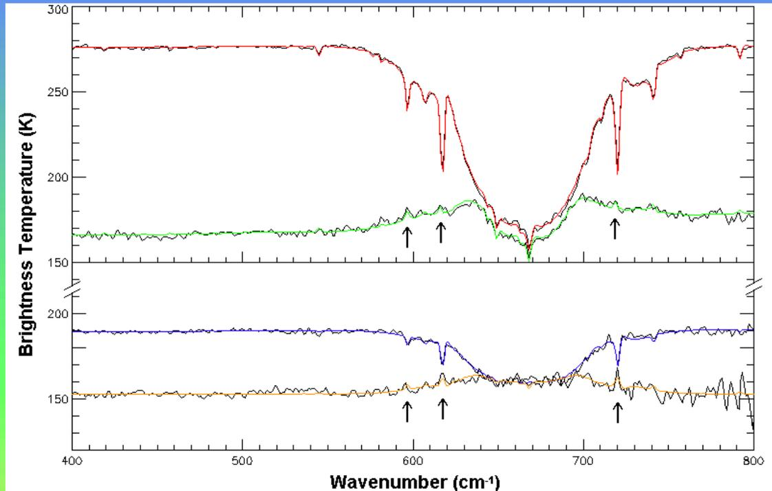
Typical quality of PFS spectra modeling for different thermal conditions of the atmosphere. *Black curves*: single spectra measured by PFS. *Colored curves*: synthetic spectra.
