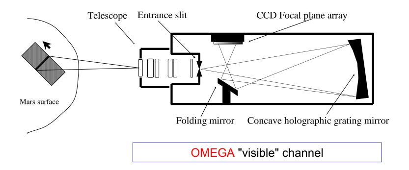
One line of 128 pixels at the surface of Mars is imaged at once, and spectrally dispersed along the other dimension of the matrix.
